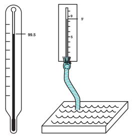
**Figure 1.** A wet-bulb thermometer is easily made using a dry thermometer. The wet bulb registers a lower temperature than the dry bulb because evaporation cools the thermometer. The wet-bulb reading is an index of relative humidity.
